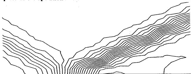
Fig. 2c Pressure contours—shock reflection problem: normal momentum pressure extrapolation.
